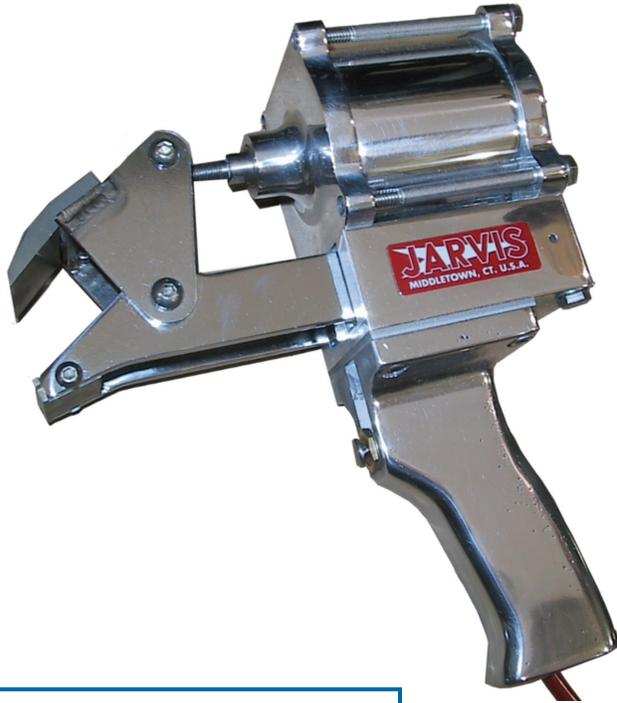
**The Jarvis Model PFC-1 - pneumatically powered picking finger cutter.**
