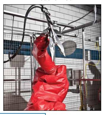
The Jarvis Model JR-50 Robotic Beef and Hog Hock Cutter for automatic hock cutting operations on the kill floor.
