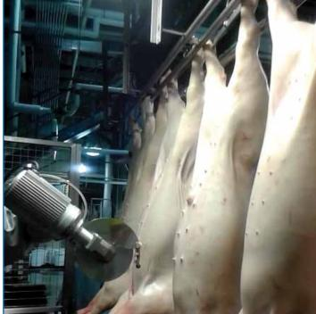
The Jarvis Model JR-50 Belly Ripper for automatic pork belly cutting operations on the kill floor.
