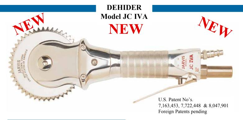
The Jarvis Model JC IVA - pneumatically powered dehider.
