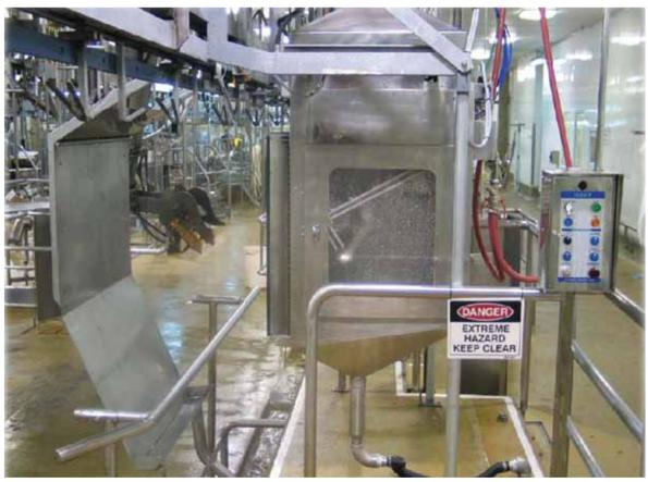
The Jarvis Model ABS-1 - hydraulic operated automatic brisket saw for sheep.
